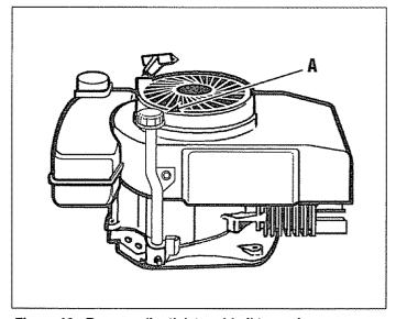
Figure 18: Remove dipstick to add oil to engine.
